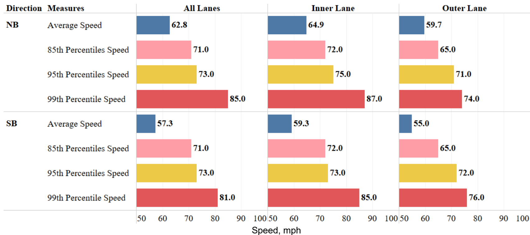
Figure 11 Speed Distribution by Lane and Direction at Work Zone 6 (Work Zone Speed Limit: 55 mph; Sample Size: 33,596 (NB) and 33,116 (SB))
