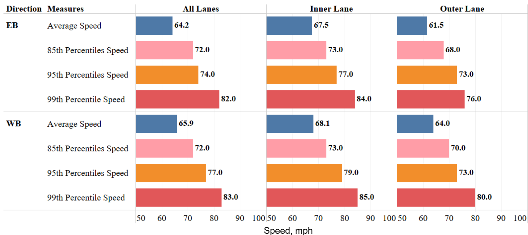
Figure 9 Speed Distribution by Lane and Direction at Work Zone 4 (Work Zone Speed Limit: 55-65 mph; Sample Size: 27,040 (EB) and 25,457 (WB))
